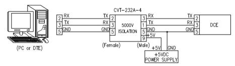
FIGURE 1: CVT-232A-4 CONNECTION DIAGRAM (DTE TO DCE)
