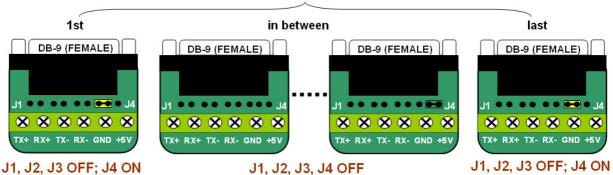
Turn on the  $120\Omega$  end-of-line terminator on both ends of the RS-485/RS-422 bus when the data rate is over 19.2kbps or the RS-485/RS-422's distance exceeds 660ft (200m).
