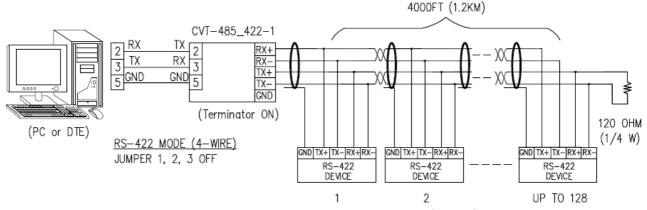
FIGURE 2: MASTER-SLAVE MULTI-DROP CONNECTIONS (RS-422)
