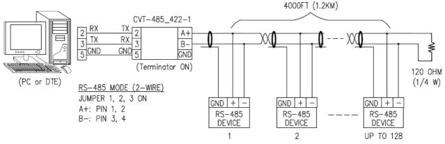
FIGURE 1: MASTER-SLAVE MULTI-DROP CONNECTIONS (RS-485)
