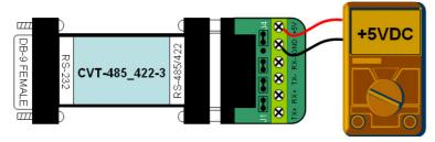
• Perform a loopback test by using CommFront's 232Analyzer software: Remove Jumper 1 and terminate Jumper 2 and 3 (or remove Jumper 1, 2, and 3 then connect TX+ to RX+ and TX- to RX-), then send commands from the 232Analyzer software. You should receive an echo of the commands sent. By performing a simple loopback test like this, you can test both the transmitter and receiver of the converter. This is very helpful when you are in doubt about the performance of your converter.
