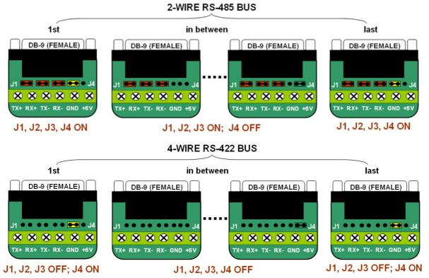
Turn on the  $120\Omega$  end-of-line terminator on both ends of the RS-485/RS-422 bus when the data rate is over 19.2kbps or the RS-485/RS-422's distance exceeds 660ft (200m).
