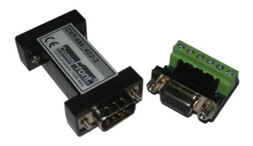
Industrial Port-Powered RS232 ⇔ RS422/RS485 Isolated Converter (Part Number: CVT-485\_422-3)
