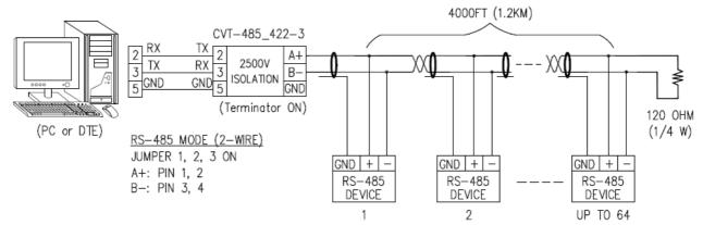
FIGURE 1: MASTER-SLAVE MULTI-DROP CONNECTIONS (RS-485)
