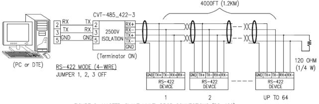
FIGURE 2: MASTER-SLAVE MULTI-DROP CONNECTIONS (RS-422)
