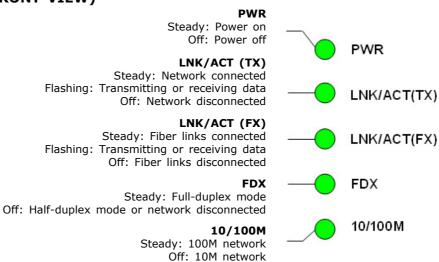
FIGURE 4: FBR-ETHERNET-2 LED INDICATIONS
