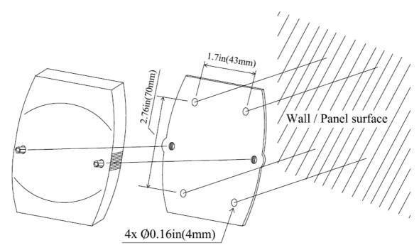
FIGURE 3: WALL/PANEL MOUNTING
