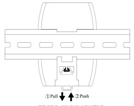
FIGURE 2: DIN-RAIL MOUNTING
