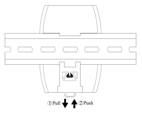
FIGURE 2: DIN-RAIL MOUNTING
