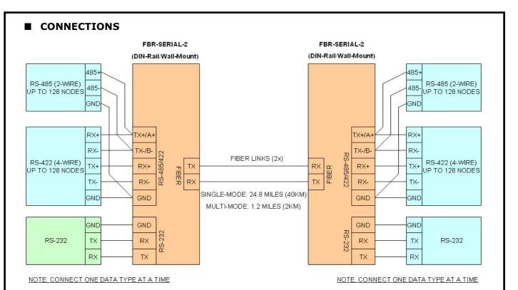
FIGURE 1: FBR-SERIAL-2 CONNECTION DIAGRAM
