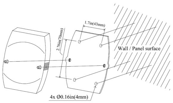
FIGURE 3: WALL/PANEL MOUNTING
