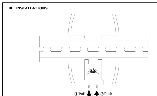
FIGURE 5: DIN-RAIL MOUNTING
