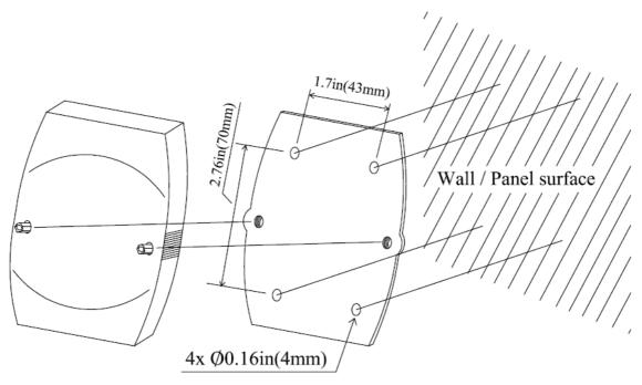
FIGURE 6: WALL/PANEL MOUNTING
