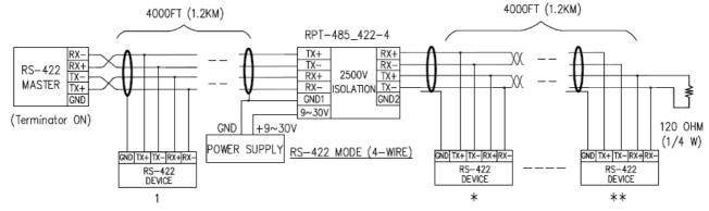
FIGURE 2: FOUR-WIRE RS-422 REPEATER
