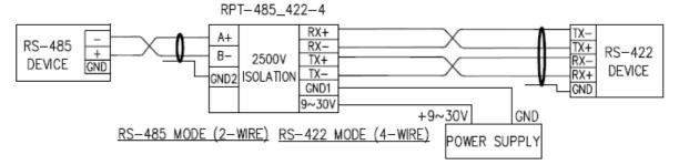
FIGURE 3: TWO-WIRE RS-485 ⇔ FOUR-WIRE RS-422 CONVERTER
