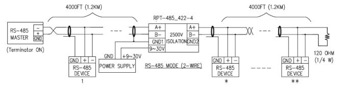
FIGURE 1: TWO-WIRE RS-485 REPEATER
