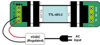
• The  $120\Omega$  end-of-line terminator adds heavy DC loading to a system; connect it only when the data rate is over 19.2kbps or the RS-485's distance exceeds 660ft (200m).
