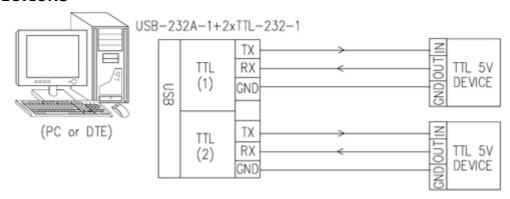
(FIGURE 1: USB-DUAL-TTL CONVERTER CONNECTION DIAGRAM)
