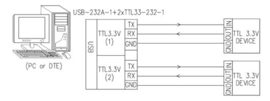
(FIGURE 1: USB-DUAL-TTL 3.3V CONVERTER CONNECTION DIAGRAM)
